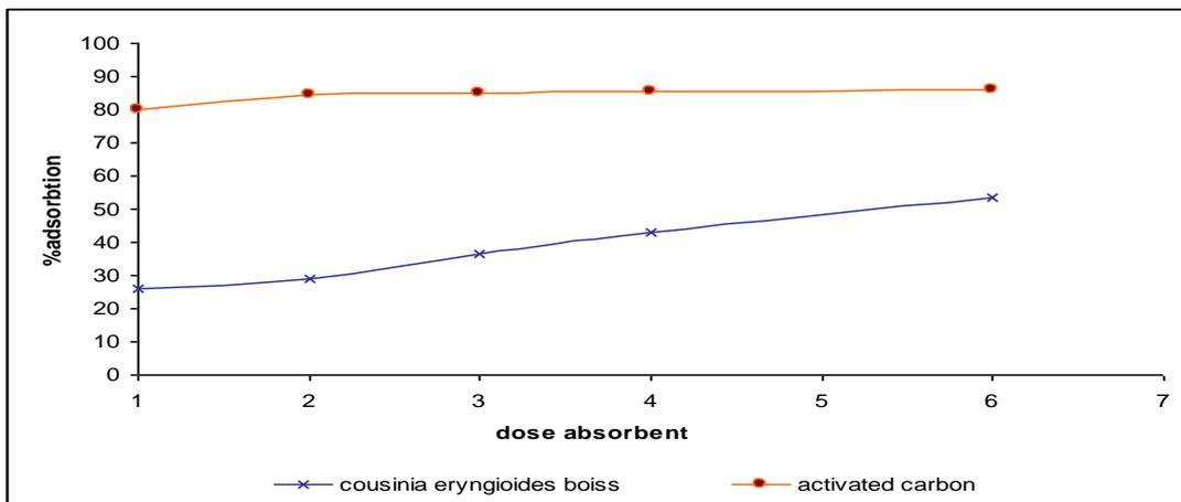
Fig. 3. Effect of dose on Cr (VI) adsorption
