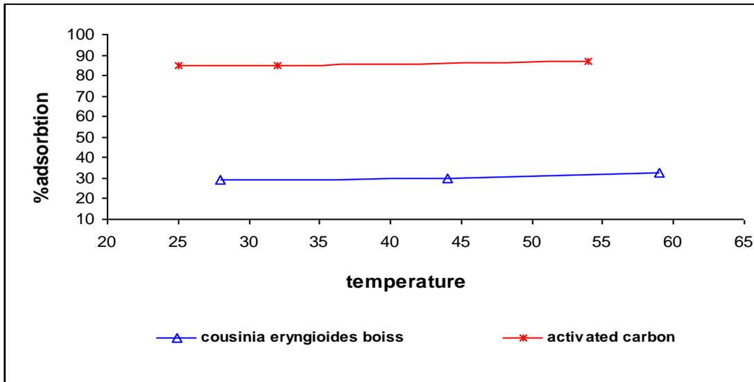
Fig. 6. Effect of temperature on Cr (VI) adsorption
