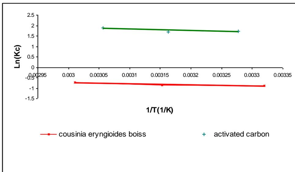
Fig. 5. Vant Hoff's plot at ambient temperature
