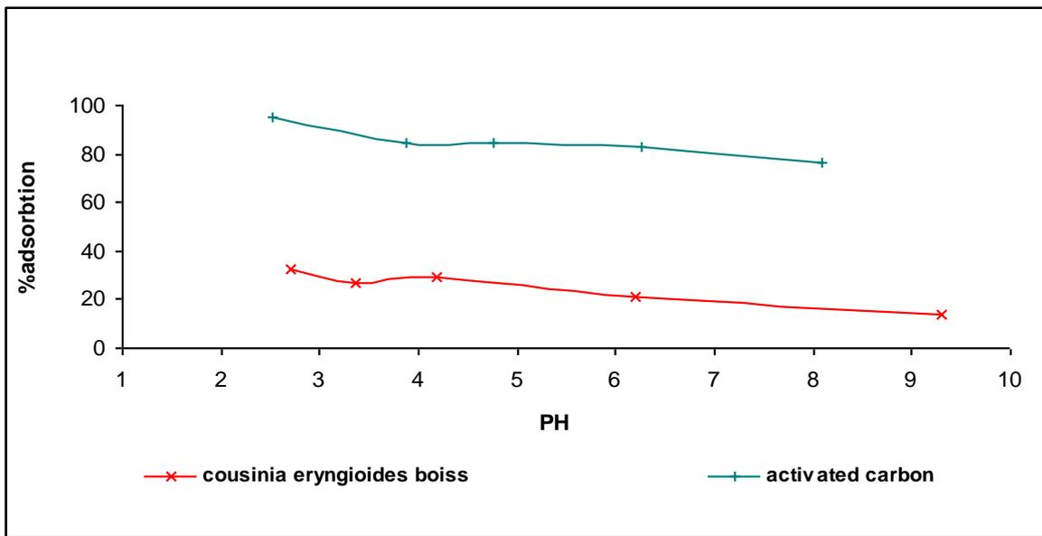
Fig. 4. Effect of PH on Cr (VI) adsorption
