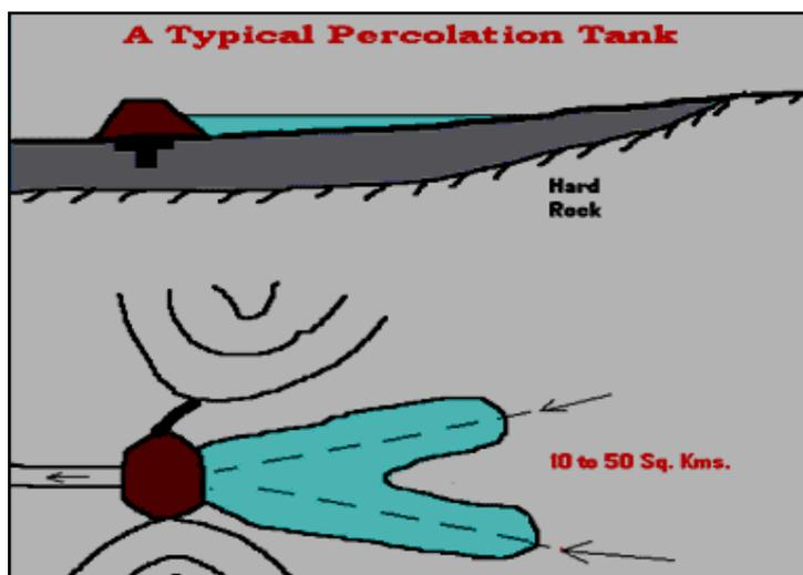
Fig. 1. Cross Section and Plan of a typical percolation tank: Earthen bund is shown in brown colour. The partial cut-off trench lies at the bottom of the bund. Water percolates from under this trench. In the plan, the waste weir is shown in black colour
