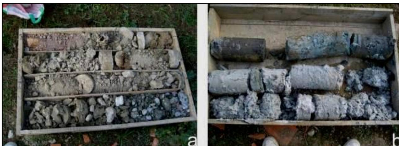
Fig. 1. Samples from the borehole; a) first four meters 0-4 m; b) core from 4-7 m.
