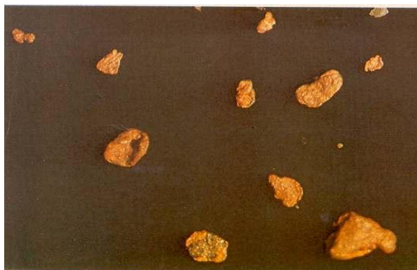
Fig.3. Darvaz (Tajikistan) Deposit: native gold from the cementing material of the conglomerates. Gold grains range from 0.5-3.0 mm, sometimes up to 5.0 mm.
