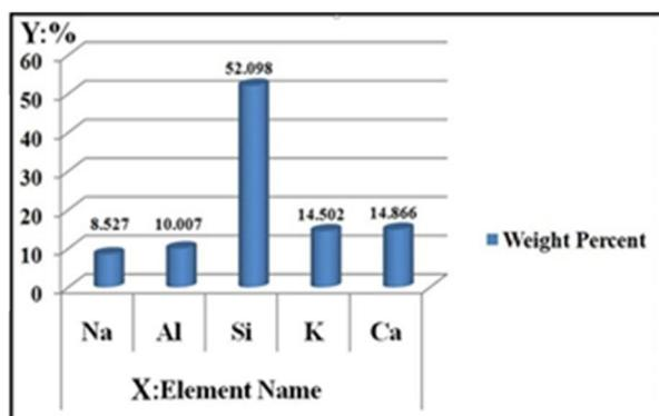
Fig.3. The comparison of SEM element analysis of Damavand zeolite.
