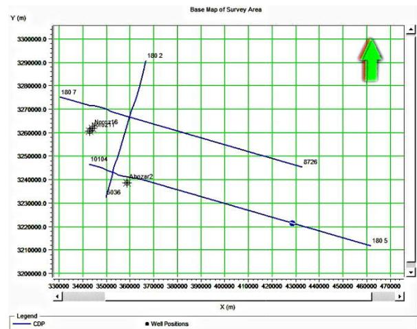
Fig. 2. A 2D Map showing the location of wells and 2D seismic sections across the Burgan reservoir.
