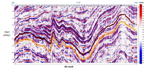
Fig. 3. 2D time section “5 SE-NW” showing the general quality of seismic data across the Burgan reservoir.
