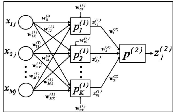
Fig. 6. A multi-layer perceptron with M inputs, K perceptrons, and a single output.
