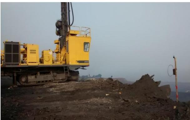
Fig 1. Personal dust monitor near drilling machine
