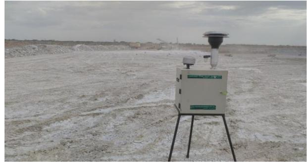
Fig 2. Ambient point dust monitor near drilling activity in limestone benches
